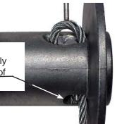
Wind on the cable by pulling in a light load to keep the tension constant. Allow the cable to swivel by using a length of chain or a swivel block between the cable hook and the load.
