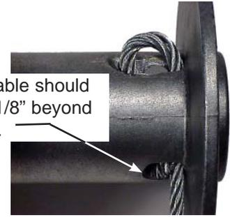
Wind on the cable by pulling in a light load to keep the tension constant. Allow the cable to swivel by using a length of chain or a swivel block between the cable hook and the load.
