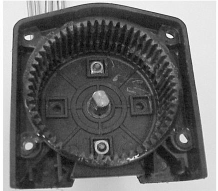
6. Replace the gears into the motor end housing, fitting the input sun gear over the motor shaft. The planetary gear carrier should be seated so that the bushing, as shown at lower right, is flush with the ring gear.
