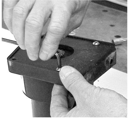
4. Lean the motor end and loosen the motor tie bolts off the tie bolt nuts. Lean the motor end back up so that it is sitting upright. **Do not let the motor end cap come apart from the rest of the motor.** Lift the motor end housing and rotate 90°. Put the tie bolt nuts in the other set of pockets and carefully lean the motor end back. Tighten the tie bolts to 45-50 in-lbs. torque. Do not over-tighten.
