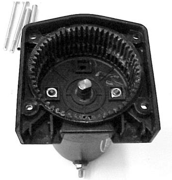
5. After rotating the motor, the motor end will appear as shown at right. The motor studs will be aligned horizontally, and the motor tie bolt nuts will be in the other set of pockets.
