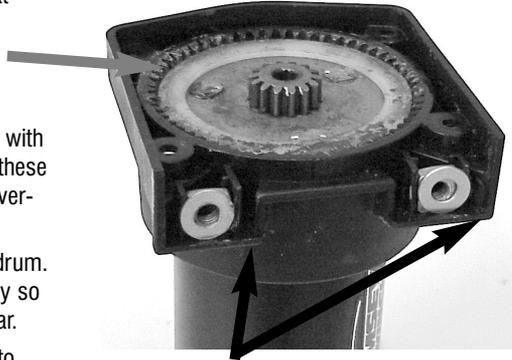
7. Re-install the end plate on the housing with the bolts you removed earlier. Tighten these bolts to 45-50 in-lbs. torque. Do not over-tighten.
