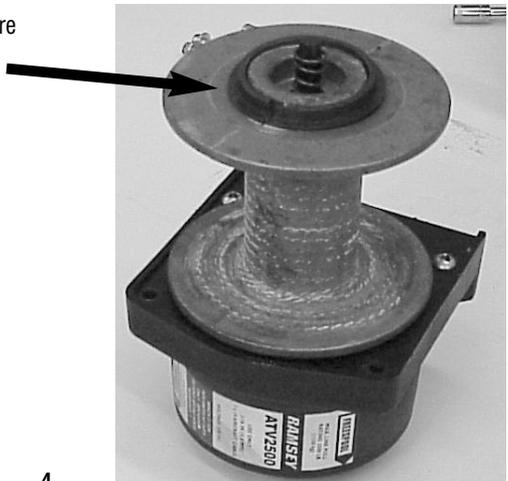
3. Remove the bolts that hold the end plate to the motor end housing. Lift off the end plate and take the nuts and washers out of the mounting feet. Set aside the gear assemblies and bushing. The input sun and planetary gear carrier may come out together.
