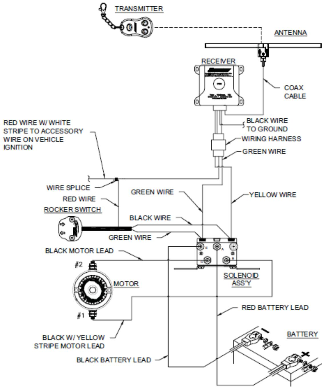
**For certain mounting applications,** where the solenoid needs to be mounted at the rear of the vehicle, switch the battery and motor leads. In this case, connect the black w/yellow stripe lead to the positive (+) terminal of the battery, and the longer black lead to the negative (-) terminal. Connect the red lead and the shorter black lead to the motor terminals.
