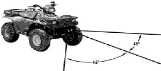
Winches equipped with cable guide fairleads can pull from several directions. Pull from an angle only to straighten up the ATV—otherwise you can damage structural members or other parts of the ATV and cause excess cable buildup on one end of the winch drum.
