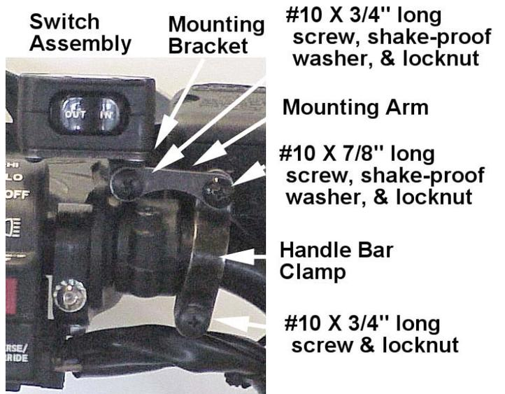
3. Install (2) Handle Bar Clamps (item #18-2) around ATV handle bars at a convenient location. Use a 3/4" long #10 screw (item #18-11) and #10 locknut (item #18-3) to secure them. See figure below and at right. Secure loosely, do not tighten.
