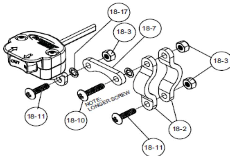
4. Install the Mounting Arm (item #18-7) to the Handle Bar Clamps using a 7/8" long #10 screw (item #18-10), shake-proof washer (item #18-17), and locknut (item #18-3). Install the shake-proof washer between the handle bar clamps and the mounting arm. Do not tighten.
